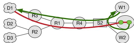
Fig. 7. The mixed (red) traffic (attack + normal requests) from  $D1$  is redirected to the  $NFV$  host which has two VNFs chained, first an IDS that monitors the traffic, finally an CAPTCHA blocker that prevents malicious requests to pass and normal traffic (green) to continue to web services ( $W1-W2$ ). (For interpretation of the references to colour in this figure legend, the reader is referred to the web version of this article.)
