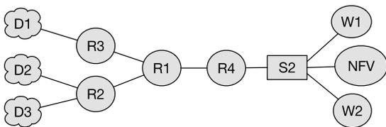
Fig. 6. Topology of the virtual network: Three domains ( $D1-D3$ ) are connected via multiple routers ( $R1-R4$ ) and a switch ( $S2$ ) to two web services ( $W1-W2$ ).  $NFV$  is a host that runs our security VNFs.
