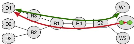
**Fig. 8.** The mixed (red) traffic (attack + normal requests) from  $D1$  is redirected to the NFV host which has two VNFs chained, first an IDS that monitors the traffic, finally a honeypot that can monitor attack behaviour. In this case normal requests (green) pass through untouched to ( $W1$ – $W2$ ). (For interpretation of the references to colour in this figure legend, the reader is referred to the web version of this article.)
