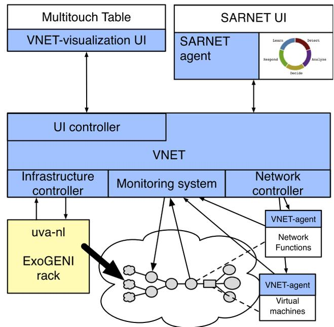
Fig. 4. Software components in the VNET prototype.
