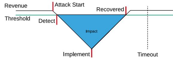
**Fig. 2.** Here, a recovery takes place. Impact: the amount of the lost revenue between the detection time and the recovery time (blue area). (For interpretation of the references to colour in this figure legend, the reader is referred to the web version of this article.)
