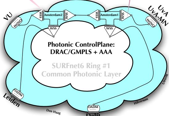
Computing nodes from the academic cluster DAS-3 can connect to the photonic portion of SURFnet6 using different logical network topologies that satisfy the needs of the application at hand: the application requests a topology through the Starplane management plane, which in turn -constraints permitting- will instruct the appropriate devices to reconfigure.
