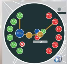
A user can modify stream forwarding of a node by zooming in on the specific node and modify its forwarding graph. For example, a rate limiter can be added to a specific path in the graph to limit its bandwidth usage.
