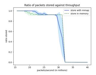
Fig. 6. Percentage of packets stored with a given amount of packets per
